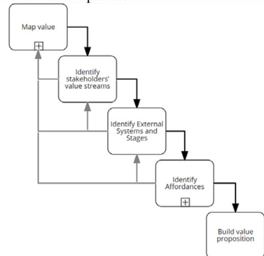
Figure 2 Building value Proposition for systems and services by adapting affordance-based design – method process
